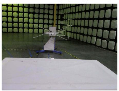
1.2 Restricted Band Around Fundamental Frequency Test Setup
