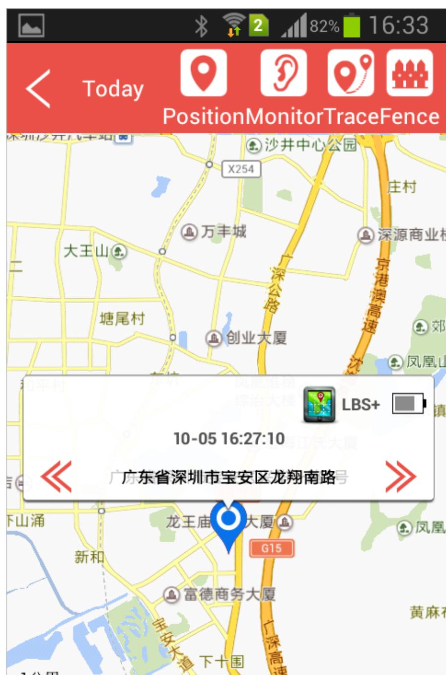
GPS indicates satellite positioning; LBS+ indicates cellular and WIFI positioning.
