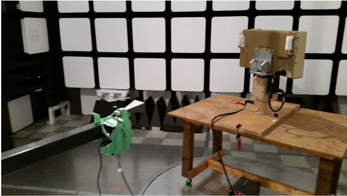
Radiated Emissions 18 GHz to 26 GHz scan
