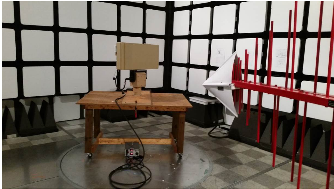
Radiated Emissions – 30 MHz to 1 GHz – Scan
