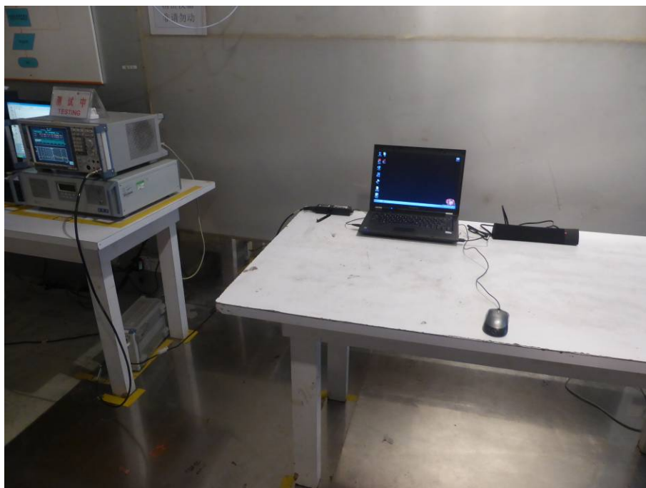
Conducted spurious emission Test Setup
