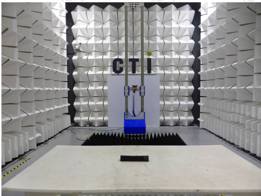
Radiated spurious emission Test Setup-2 (Above 1GHz)
