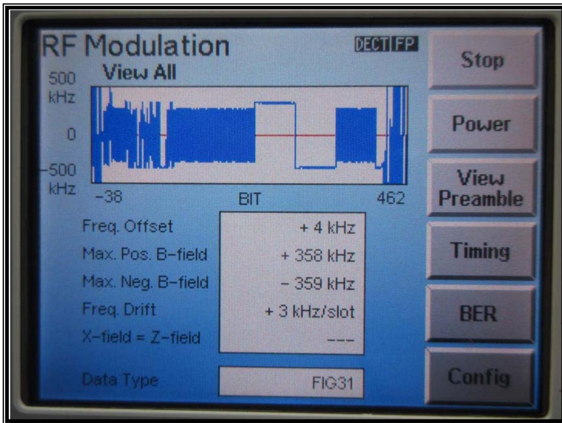
**b) Carrier Frequency Stability over power supply voltage**
