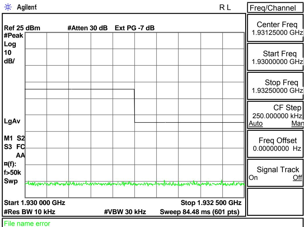
Out-of-band Unwanted Emissions: CH F<sub>L</sub>
