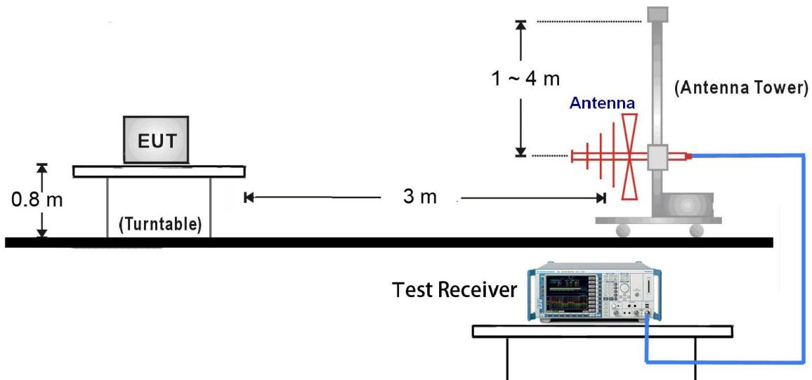
1GHz ~ 18GHz Test Setup:
