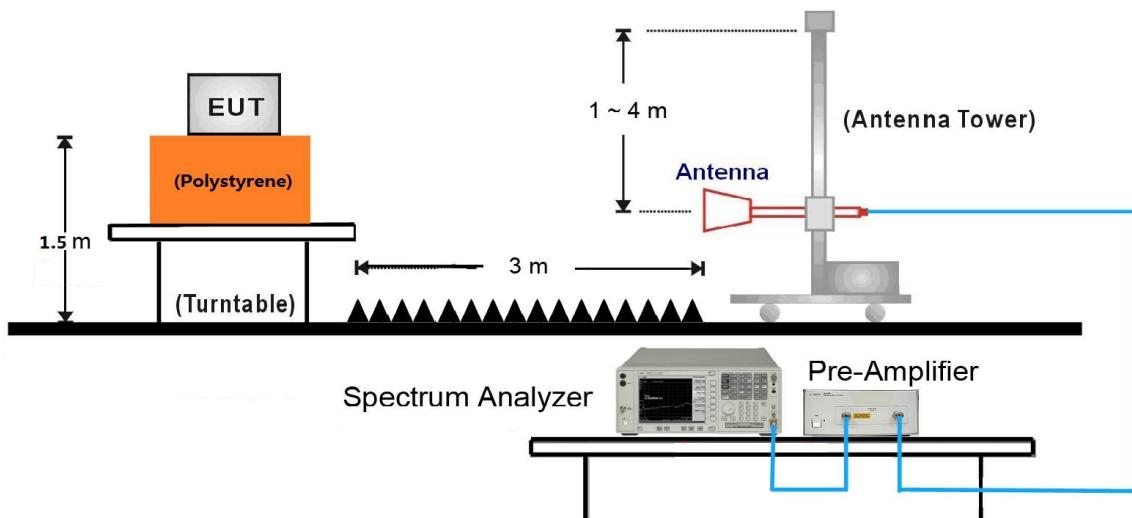
18GHz ~25GHz Test Setup:
