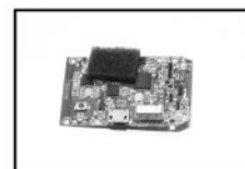
H107D+-07 Receiver PCBA board
