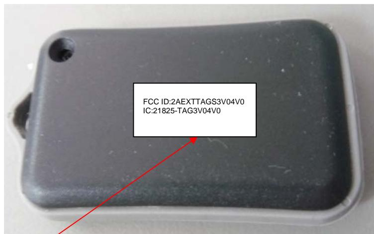
Label with **FCC ID:2AEXTTAGS3V04V0** and **IC:21825-TAG3V04V0** is located at the rear side panel of the tag. The statement according to FCC part 15 §15.19(a)(3) is placed in User manual, page 2 (Application exhibit User\_manual\_28484).
