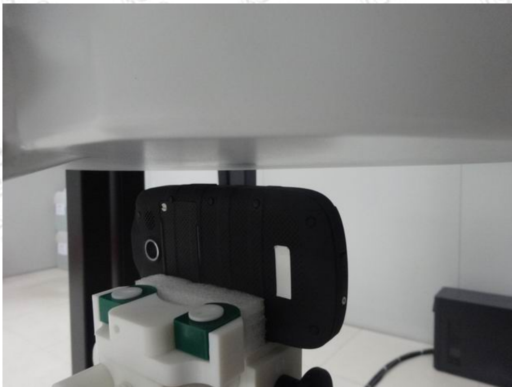
10mm body-worn Left Side Setup Photo(hotspot)
