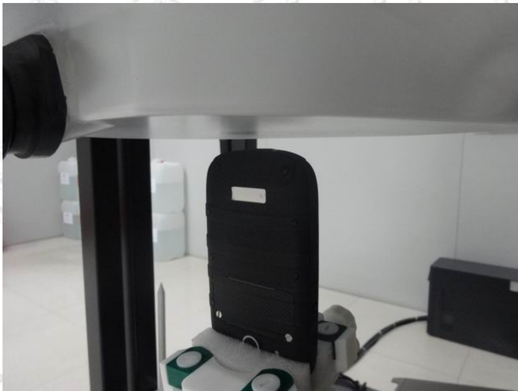
10mm body-worn Bottom Side Setup Photo(hotspot)
