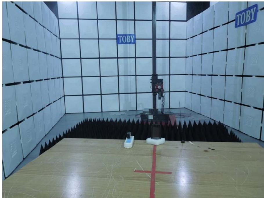
**Photo of Setup for Radiated Emission (Below 1 GHz)**
