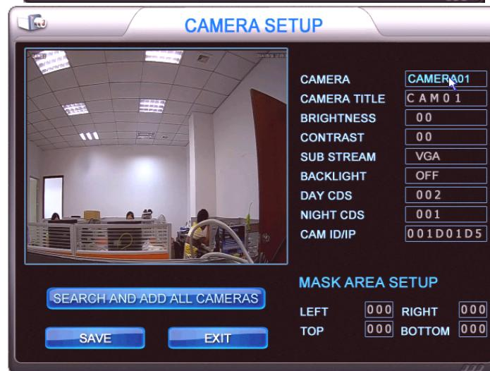
Select deferent channel, use mouse wheel to change CAM IP/ID, you can input IP address or ID number.
