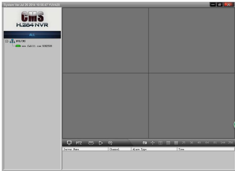
After run the software, device list window will display all NVR in local network, right click NVR/CMS, click "turn off NVR auto search", will stop auto search NVR function; Select NVR device, right click, click "Connect", if NVR and PC is same network segment, CMS will display NVR image.
