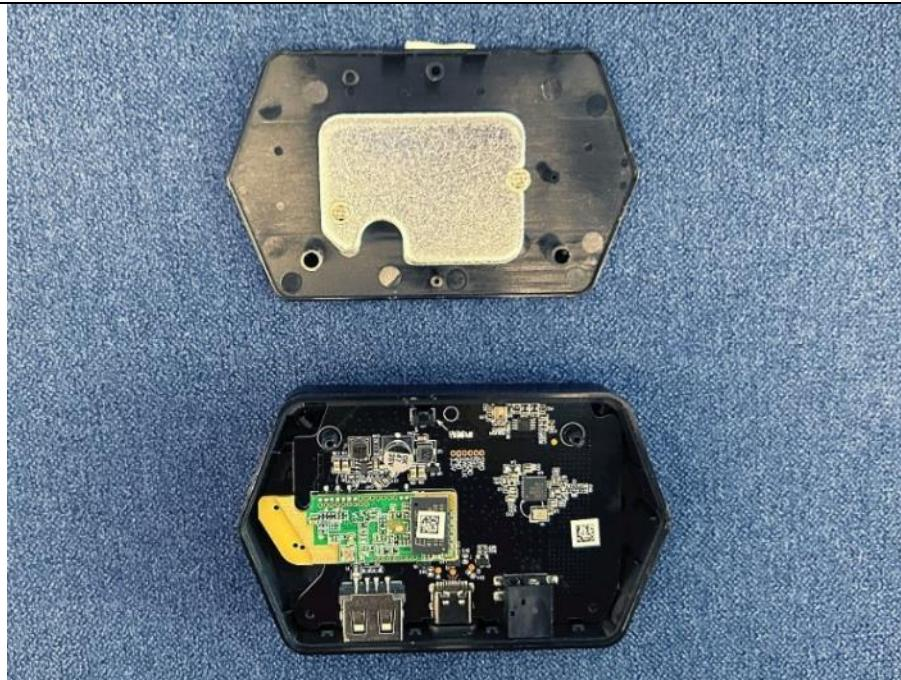
Details of: Controller PCB view
