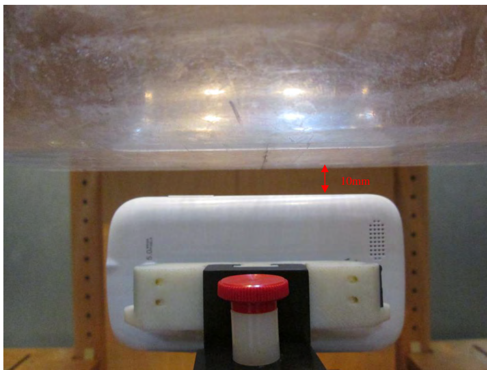
Body-worn Left Setup Photo (10mm)
