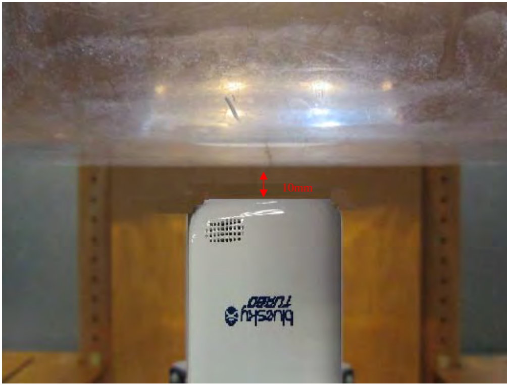
Body-worn Bottom Setup Photo (10mm)
