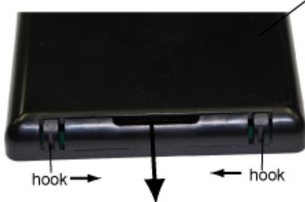
push both hook towards the middle, and pull the battery compartment out for batteries replacement
