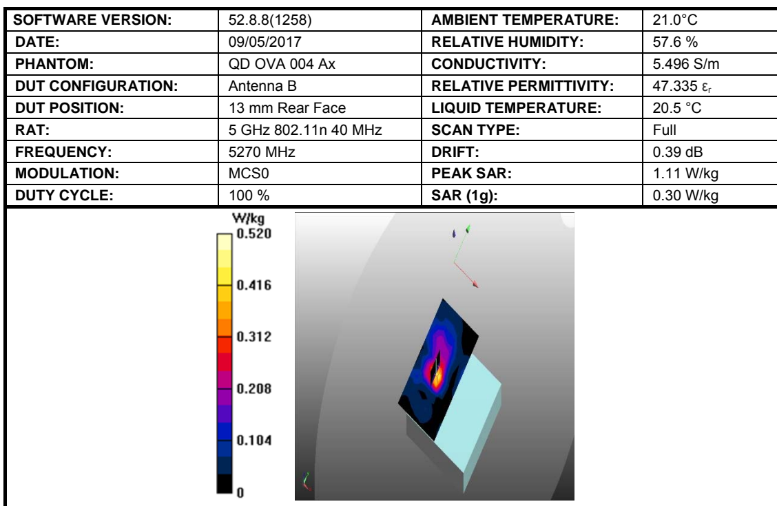
Figure 08: SAR Body Testing Results for the DAQRI Compute Pack at 5270 MHz.
