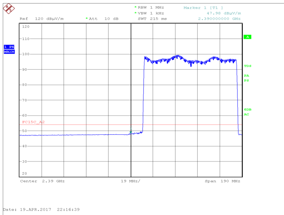
Figure 37 - Hopping - GFSK - 2402 MHz - Measured Frequency 2390.0 MHz - Average
