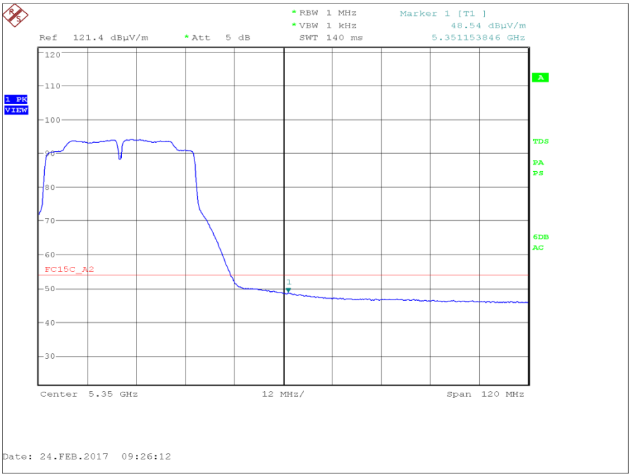
Figure 187 - U-NII 2a - Restricted Band Edge at 5350 MHz - Average
