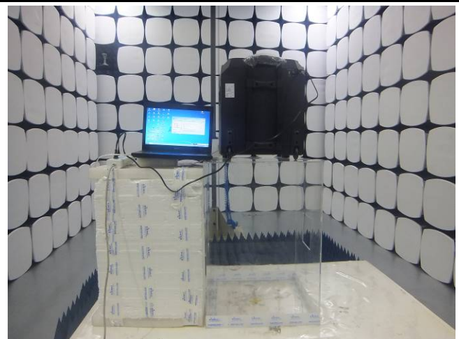
Radiated Spurious Emissions Test Above 1GHz
