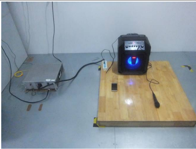
Conducted Emissions Test Setup – Front View
