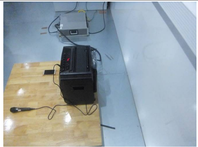
Conducted Emissions Test Setup – Side View
