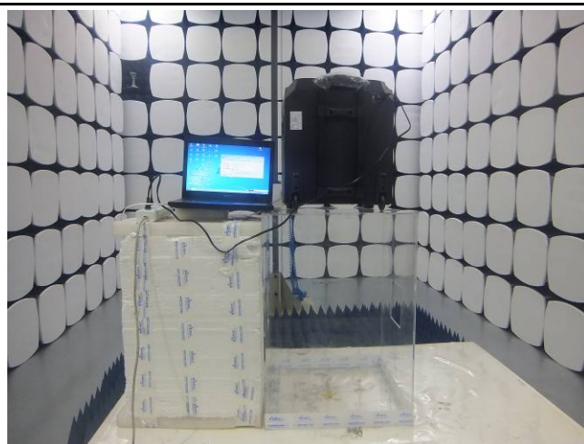
Radiated Spurious Emissions Test Above 1GHz
