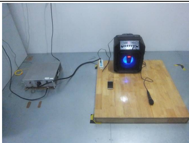
Conducted Emissions Test Setup – Front View
