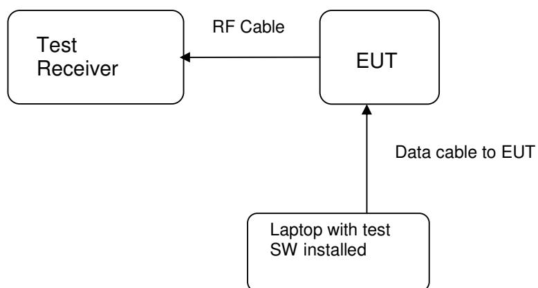
**Diagram of Measurement Equipment Configuration for AC Mains Conducted Emission Test (if applicable)**
