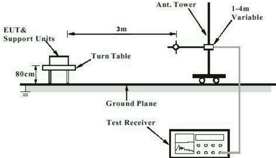
Note: For measurements above 1 GHz, there is RF absorbing material on the floor of the test site for above 1GHz measurement.
