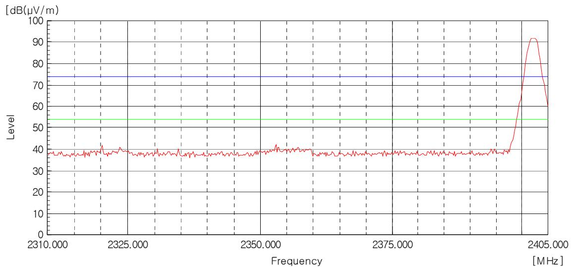
AV Detector: RBW: 1 MHz, VBW: 10 Hz (2 310 MHz - 2 390 MHz), Worst case (Low, Horizontal)
