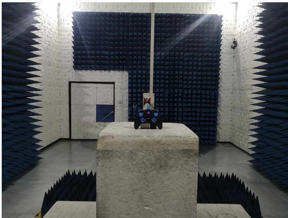
FCC RADIATED EMISSION TEST SETUP ABOVE 1GHZ
