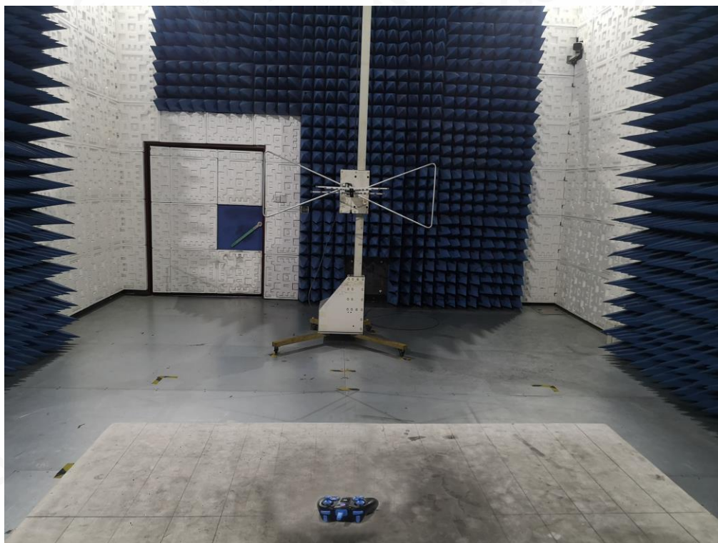
FCC RADIATED EMISSION TEST SETUP ABOVE 1GHZ
