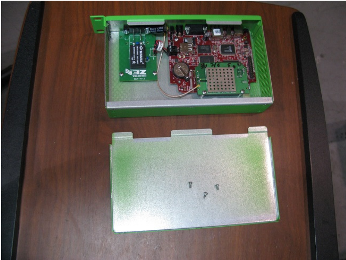
Major Components of the Data Collector: 2.4GHz Radio Board (green board plugged onto red board), Single Board Computer (red board), and DC-DC Converter Board (other green board)
