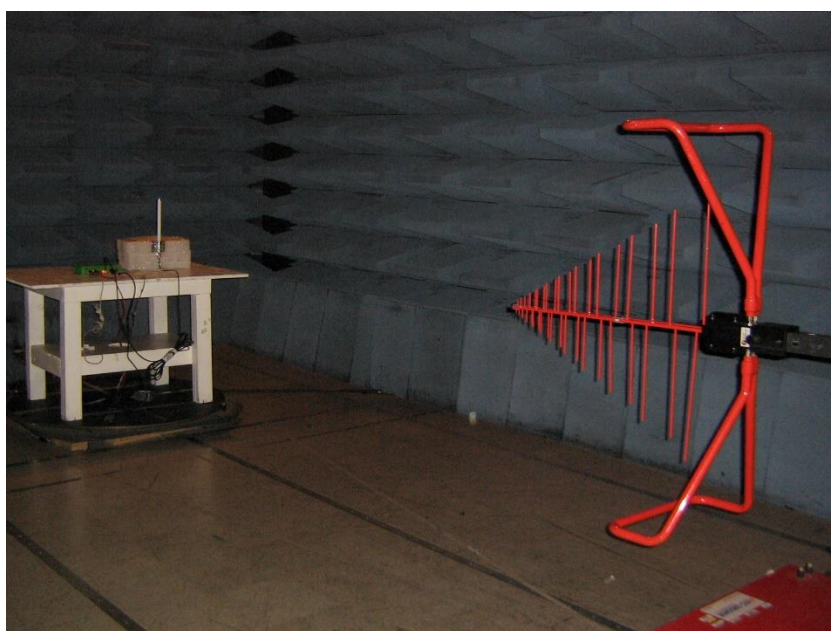
Radiated Emissions Setup in Semi-Anechoic Chamber, 30MHz -1GHz
