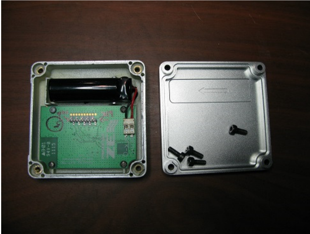
WASP Sensor Board and 3.7V/3400mAH battery installed inside enclosure
