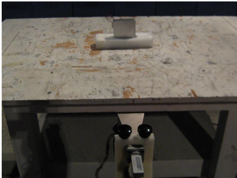
Radiated Emissions Setup in Semi-Anechoic Chamber, 18GHz-26GHz
