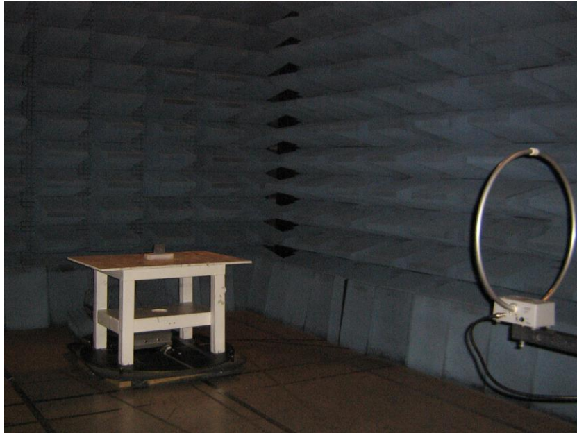
Radiated Emissions Setup in Semi-Anechoic Chamber, 150 kHz-30MHz
