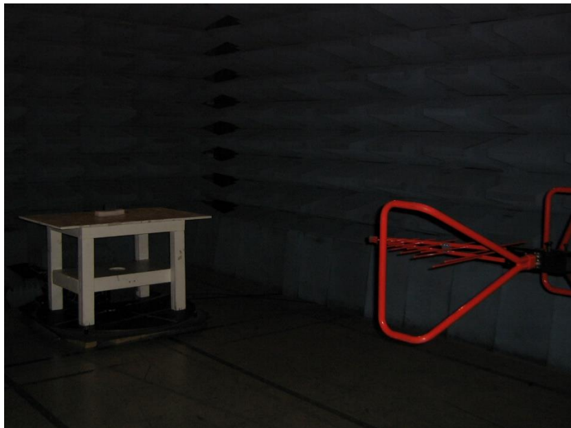
Radiated Emissions Setup in Semi-Anechoic Chamber, 30MHz-1GHz
