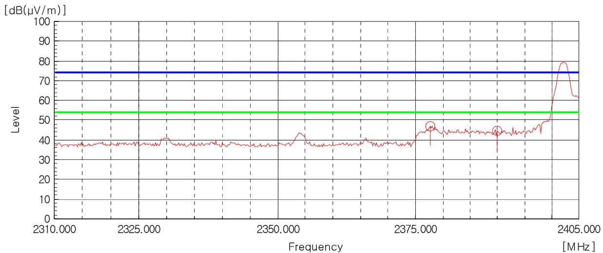
AV Detector: RBW: 1 MHz, VBW: 10 Hz (2 310 MHz - 2 390 MHz), Worst case (Low, Vertical)
