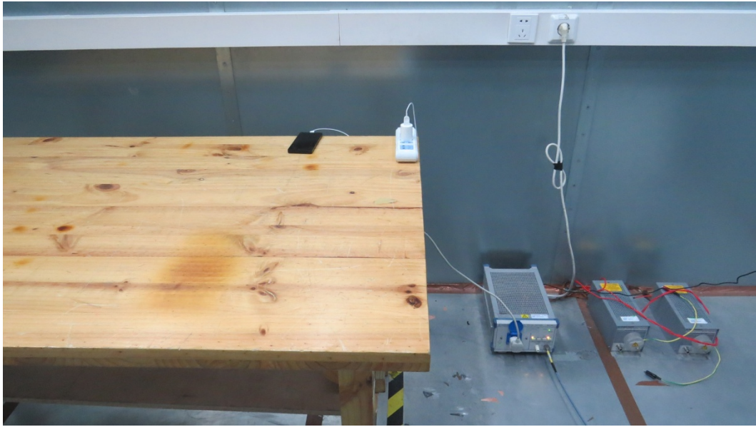
Picture 3 Conducted Emission Test Setup
