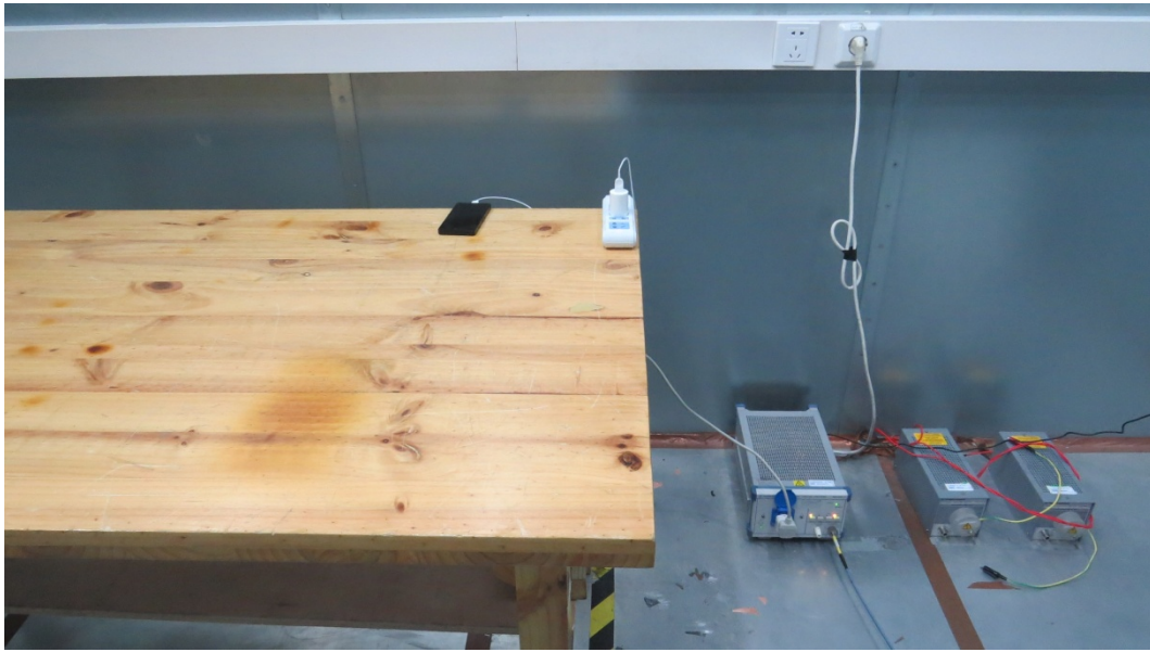
Picture 3 Conducted Emission Test Setup
