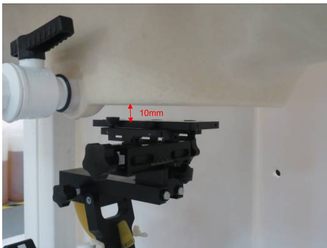
Picture 15: Back Side, the distance from handset to the bottom of the Phantom is 10mm
