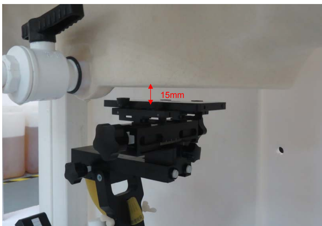
Picture 14: Front Side, the distance from handset to the bottom of the Phantom is 15mm
