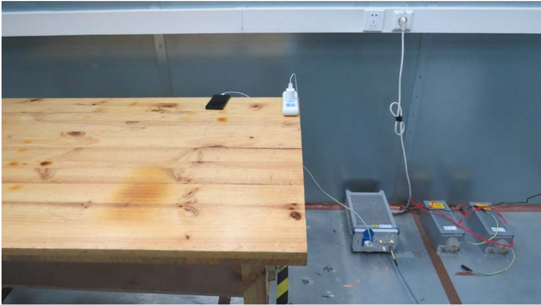
Picture 3 Conducted Emission Test Setup
