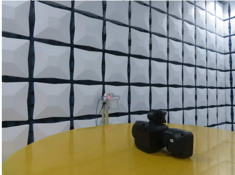
Photograph 2: Set-up for Radiated Spurious Emissions (18GHz-40GHz)
