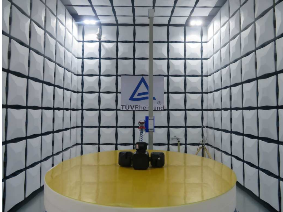
Photograph 1: Set-up for Radiated Spurious Emissions (1GHz-18GHz)
