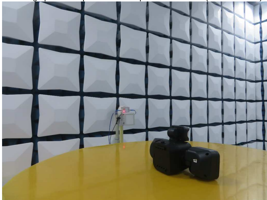
Photograph 2: Set-up for Radiated Spurious Emissions (18GHz-40GHz)
