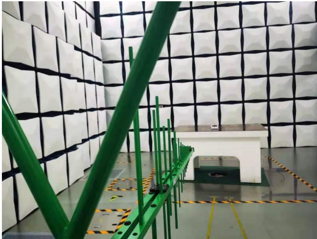
Photograph 2: Set-up for Radiated Emission, above 1GHz
