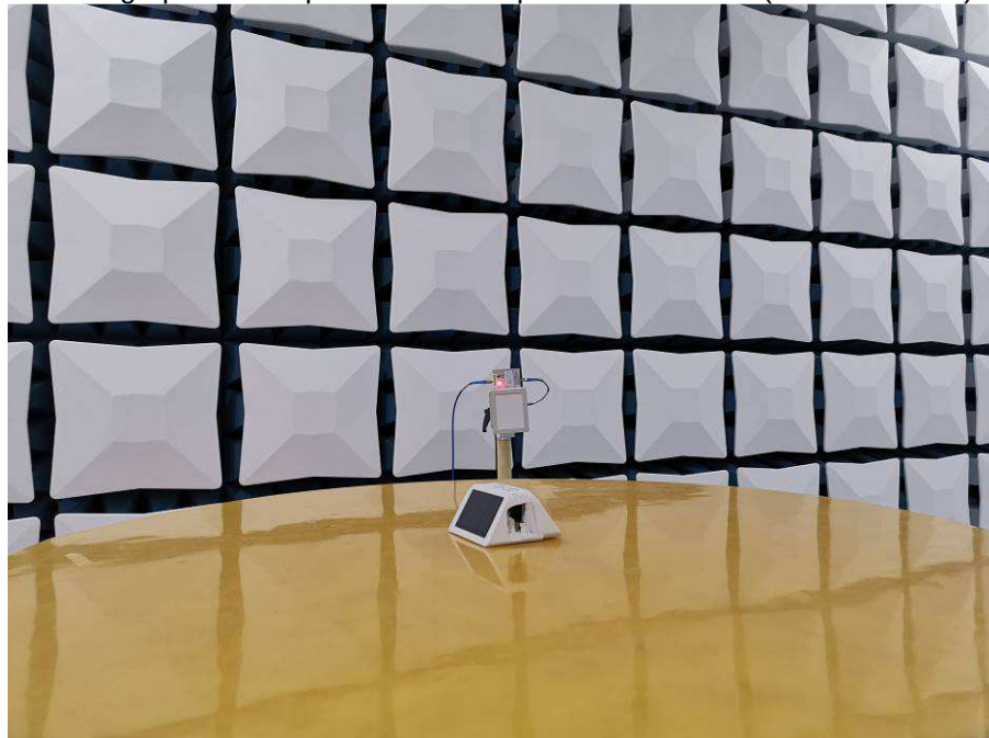
Photograph 2: Set-up for Radiated Spurious Emissions (18GHz-25GHz)
