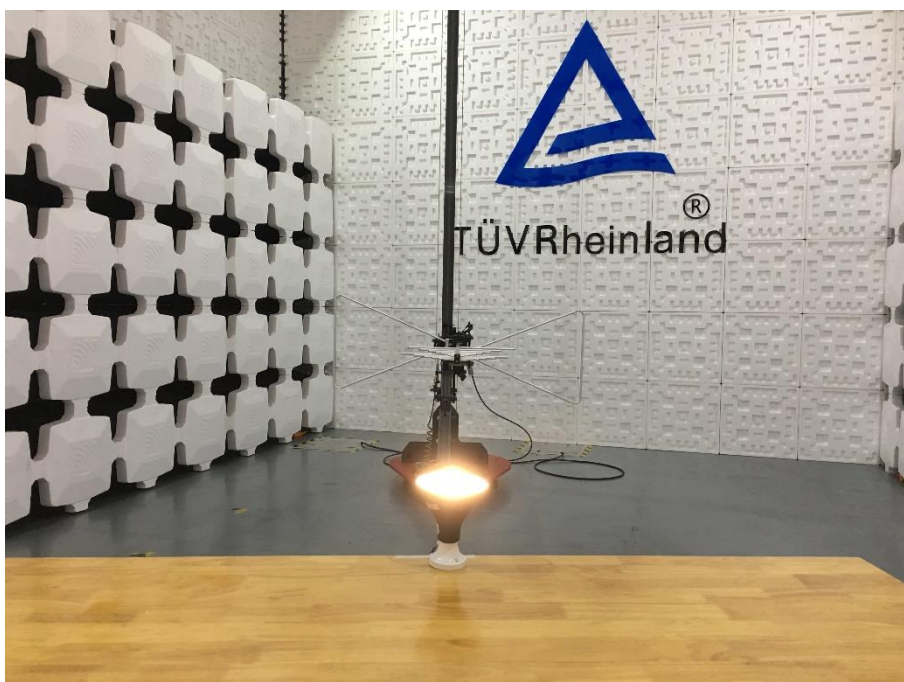
Photograph 4: Set-up for Radiated Emission, Below 1GHz
