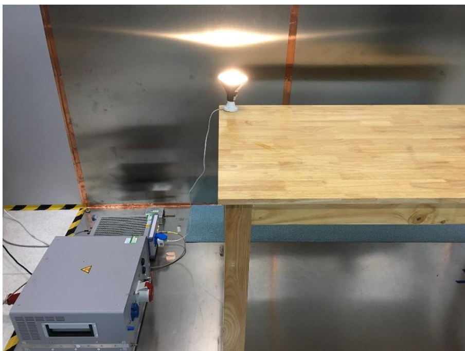
Photograph 3: Set-up for Conducted Emission on AC Mains
