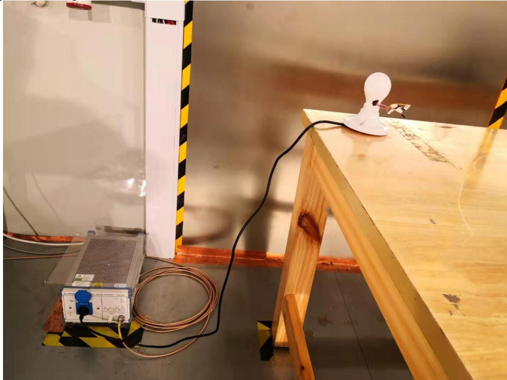
Photograph 3: Set-up for Conducted Emission
