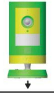
NOTE: For a downward angle, face the longer side of the base toward the front and tilt your camera down accordingly. /
