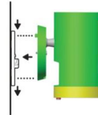
9. Unclasp the camera mount and tighten the security screw. / Unclasp the camera mount and tighten the security screw. / Unclasp the camera mount and tighten the security screw.
