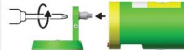
3. Slide to remove the mounting plate from the camera mount. / Slide to remove the mounting plate from the camera mount. / Slide to remove the mounting plate from the camera mount.
