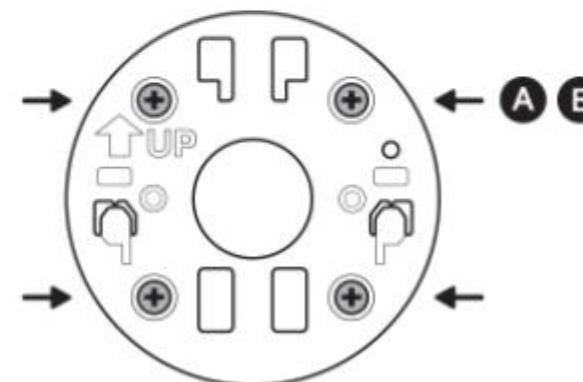
On stucco, brick, or concrete, use a 1/4 in (6 mm) masonry bit to drill holes for the included wall anchors. / On stucco, brick, or concrete, use a 1/4 in (6 mm) masonry bit to drill holes for the included wall anchors. / On stucco, brick, or concrete, use a 1/4 in (6 mm) masonry bit to drill holes for the included wall anchors.
