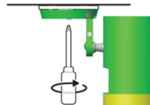
10. If installing outside, tighten the security screw on the battery cover. / If installing outside, tighten the security screw on the battery cover. / If installing outside, tighten the security screw on the battery cover.
