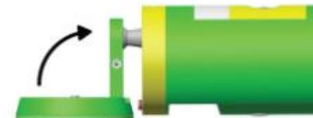
2. Unscrew to detach the camera mount from the battery cover. / Unscrew to detach the camera mount from the battery cover. / Unscrew to detach the camera mount from the battery cover.
