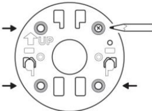
5. Install the mounting plate with the UP arrow pointing up. / Install the mounting plate with the UP arrow pointing up. / Install the mounting plate with the UP arrow pointing up.
