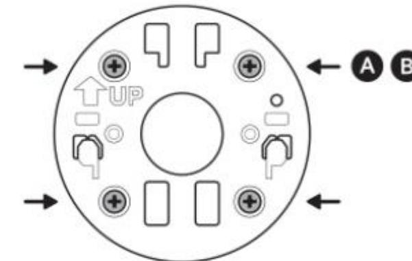
On stucco, brick, or concrete, use a 1/4 in (6 mm) masonry bit to drill holes for the included wall anchors. / On stucco, brick, or concrete, use a 1/4 in (6 mm) masonry bit to drill holes for the included wall anchors. / On stucco, brick, or concrete, use a 1/4 in (6 mm) masonry bit to drill holes for the included wall anchors.
