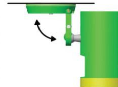
11. Adjust your camera's angle, then tighten the screw on the camera mount arm to secure in place. / Adjust your camera's angle, then tighten the screw on the camera mount arm to secure in place. / Adjust your camera's angle, then tighten the screw on the camera mount arm to secure in place.
