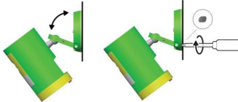
11. Adjust your camera's angle, then tighten the screw on the camera mount arm to secure in place. / Adjust your camera's angle, then tighten the screw on the camera mount arm to secure in place. / Adjust your camera's angle, then tighten the screw on the camera mount arm to secure in place.
