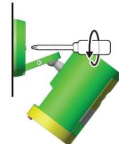
10. If installing outside, tighten the **1** security screw on the battery cover. / If installing outside, tighten the security screw on the battery cover. / If installing outside, tighten the security screw on the battery cover.
