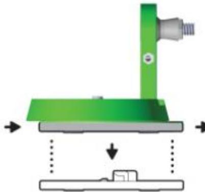
4. Use the mounting plate as a guide to mark screw holes on the wall. / Use the mounting plate as a guide to mark screw holes on the wall. / Use the mounting plate as a guide to mark screw holes on the wall.
