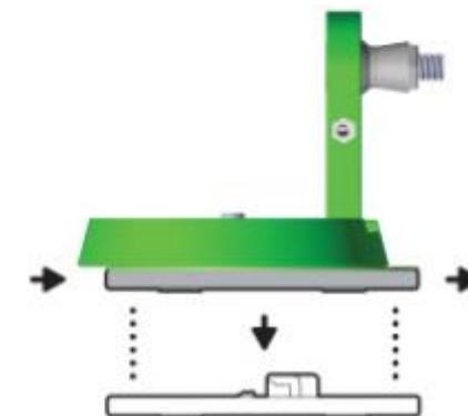
4. Use the mounting plate as a guide to mark screw holes on the wall. / Use the mounting plate as a guide to mark screw holes on the wall. / Use the mounting plate as a guide to mark screw holes on the wall.
