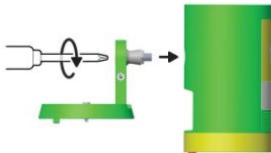
8. Clasp the camera mount and attach your camera to the mounting plate by sliding until you feel a click. / Clasp the camera mount and attach your camera to the mounting plate by sliding until you feel a click. / Clasp the camera mount and attach your camera to the mounting plate by sliding until you feel a click.
