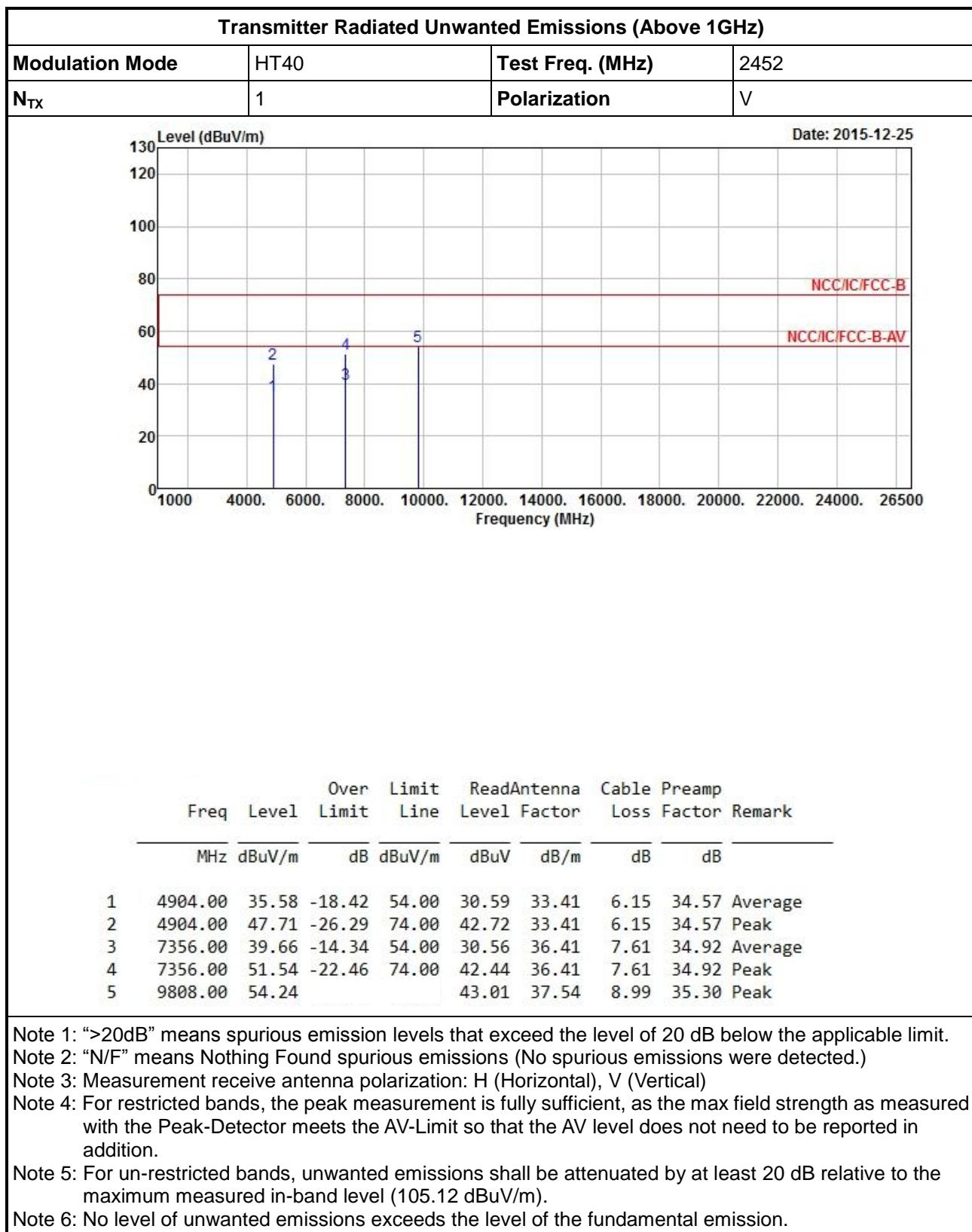
Note 1: ">20dB" means spurious emission levels that exceed the level of 20 dB below the applicable limit.
