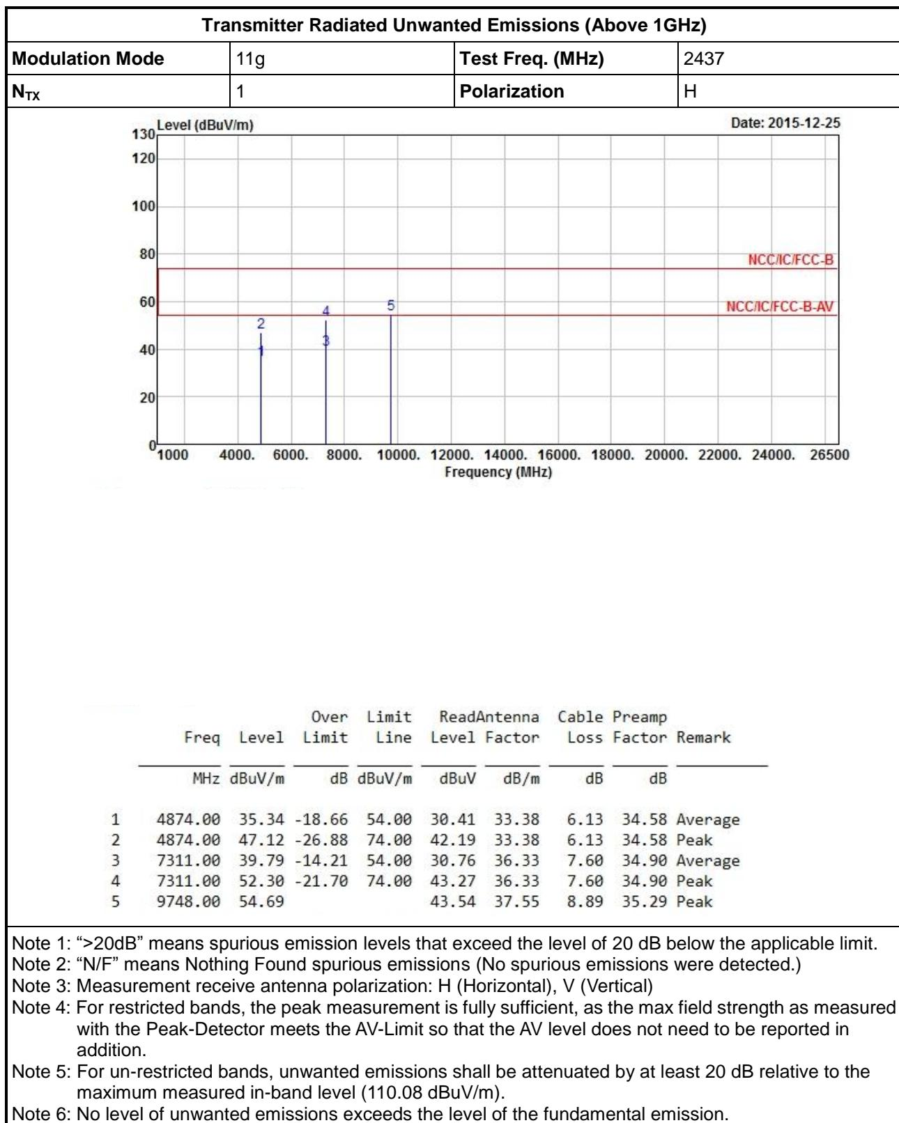
Note 1: ">20dB" means spurious emission levels that exceed the level of 20 dB below the applicable limit.
