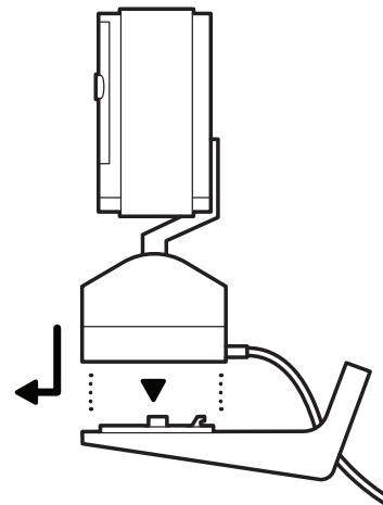
5. Secure your camera and bracket to the mounting plate by sliding until you feel a click. / *Secure your camera and bracket to the mounting plate by sliding until you feel a click. / Secure your camera and bracket to the mounting plate by sliding until you feel a click.*
