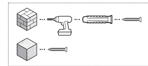
On stucco, brick, or concrete, use a 3/16 in (5 mm) masonry bit to drill holes for the included wall anchors. / On stucco, brick, or concrete, use a 3/16 in (5 mm) masonry bit to drill holes for the included wall anchors. / On stucco, brick, or concrete, use a 3/16 in (5 mm) masonry bit to drill holes for the included wall anchors.
