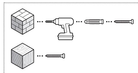
On stucco, brick, or concrete, use a 3/16 in (5 mm) masonry bit to drill holes for the included wall anchors. / On stucco, brick, or concrete, use a 3/16 in (5 mm) masonry bit to drill holes for the included wall anchors. / On stucco, brick, or concrete, use a 3/16 in (5 mm) masonry bit to drill holes for the included wall anchors.
