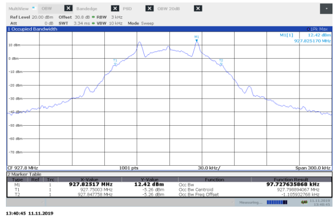
Figure 8.5-6: 99% OBW on high channel
