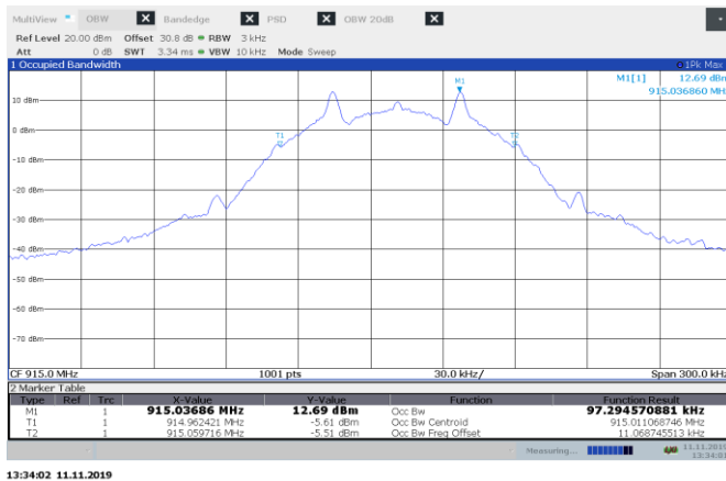
Figure 8.5-5: 99% OBW on mid channel
