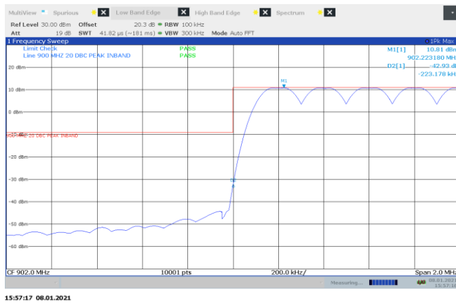
Figure 8.8-3: Conducted Low Band-edge on hopping, FSK 50kbps
