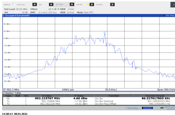
Figure 8.4-4: 99% OBW on low channel, 50 kbps
