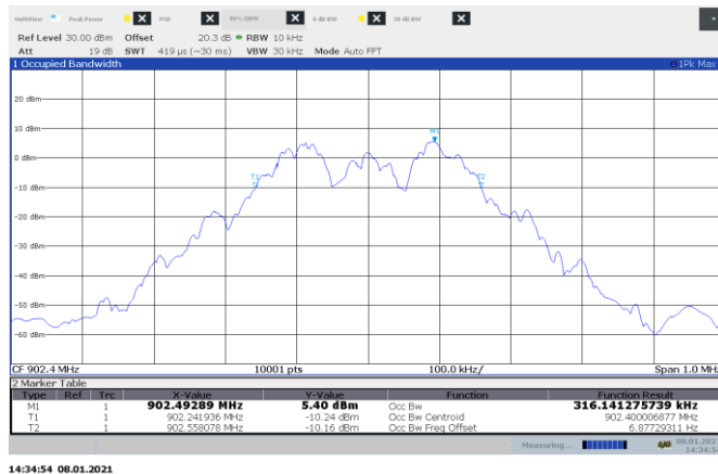
Figure 8.4-14: 99% OBW on low channel, 150 kbps
