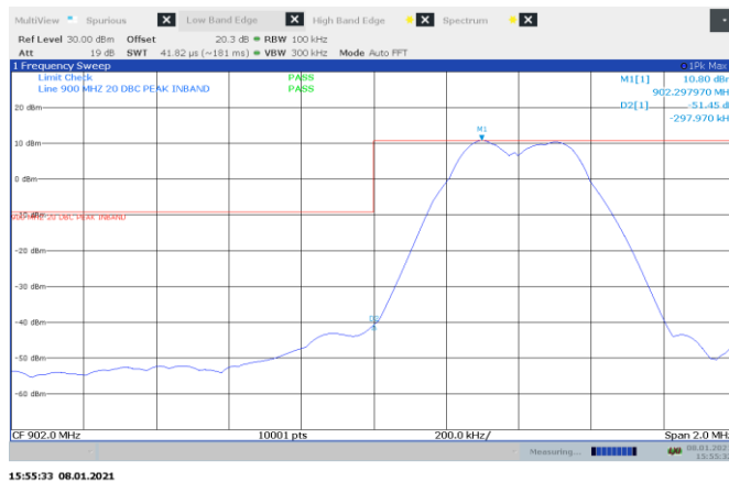
Figure 8.8-15: Conducted Band-edge on low channel, FSK 150kbps
