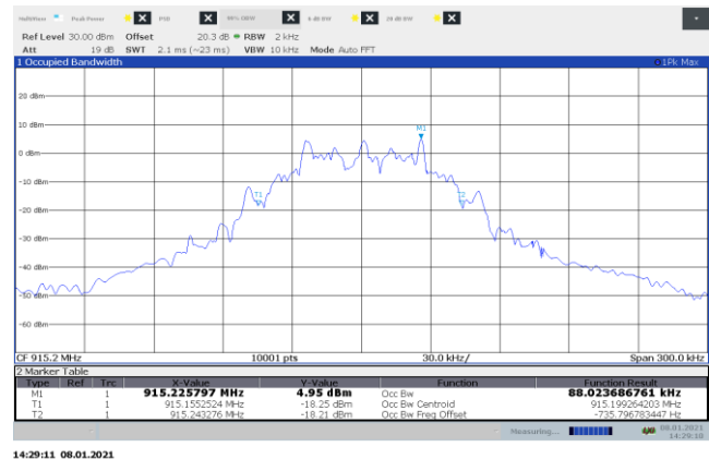
Figure 8.4-5: 99% OBW on mid channel, 50 kbps
