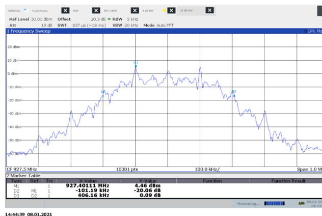
Figure 8.4-23: 20 dB bandwidth on high channel, 250 kbps
