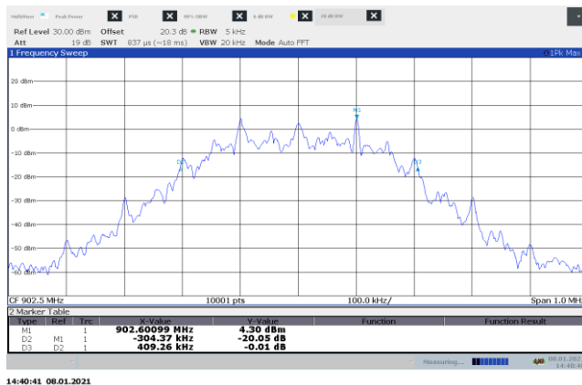
Figure 8.4-21: 20 dB bandwidth on low channel, 250 kbps
