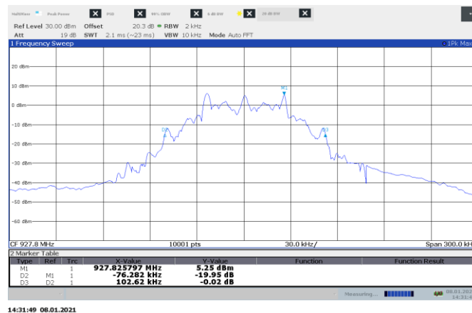
Figure 8.4-3: 20 dB bandwidth on high channel, 50 kbps
