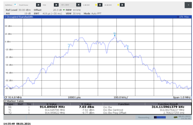
Figure 8.4-15: 99% OBW on mid channel, 150 kbps
