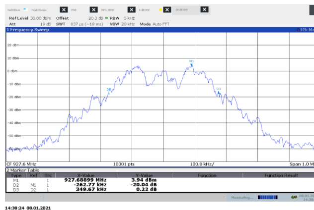
Figure 8.4-13: 20 dB bandwidth on high channel, 150 kbps
