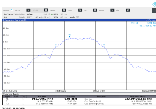
Figure 8.6-3: 99% OBW on 912 MHz channel, Z-Wave Long Range
