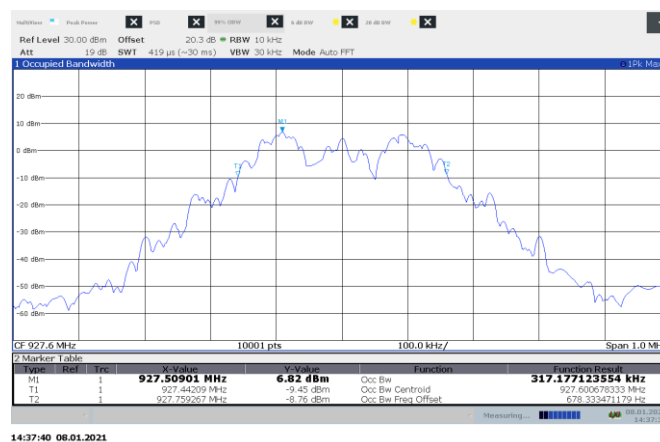
Figure 8.4-16: 99% OBW bandwidth on high channel, 150 kbps
