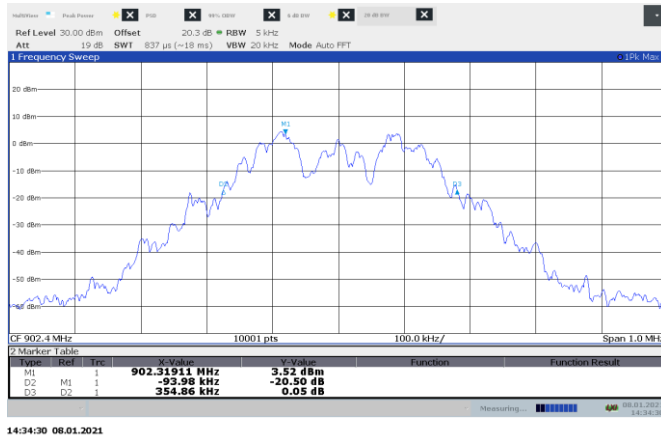
Figure 8.4-11: 20 dB bandwidth on low channel, 150 kbps
