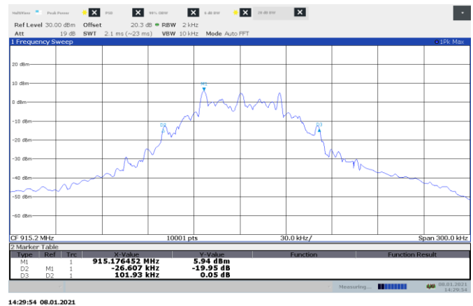
Figure 8.4-2: 20 dB bandwidth on mid channel, 50 kbps
