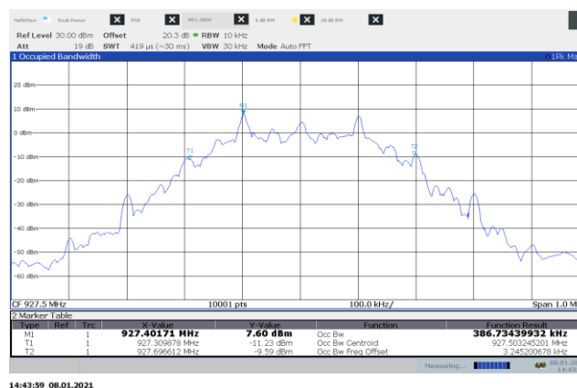
Figure 8.4-26: 99% OBW bandwidth on high channel, 250 kbps
