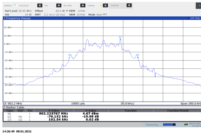
Figure 8.4-1: 20 dB bandwidth on low channel, 50 kbps
