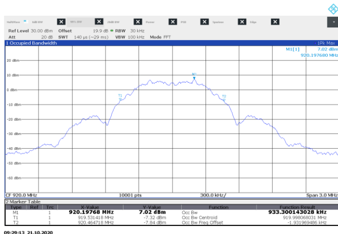
Figure 8.6-4: 99% OBW on 920 MHz channel, Z-Wave Long Range
