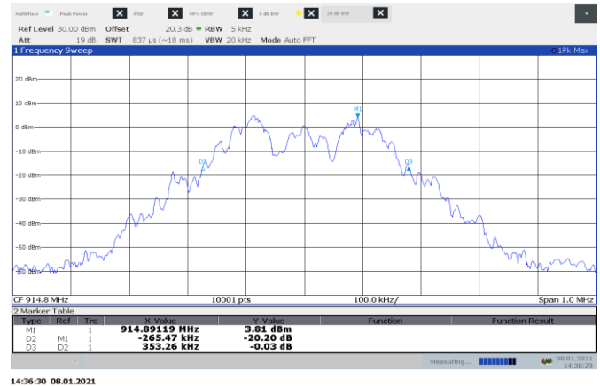
Figure 8.4-12: 20 dB bandwidth on mid channel, 150 kbps
