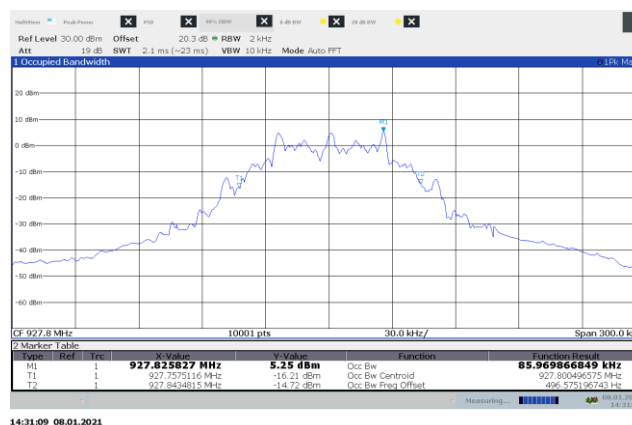
Figure 8.4-6: 99% OBW bandwidth on high channel, 50 kbps
