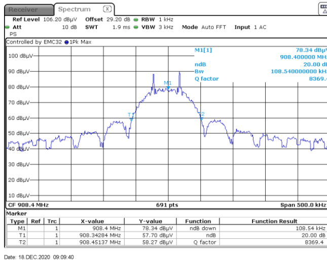
Figure 8.6-1: 20 dB occupied bandwidth, 908.4 MHz
