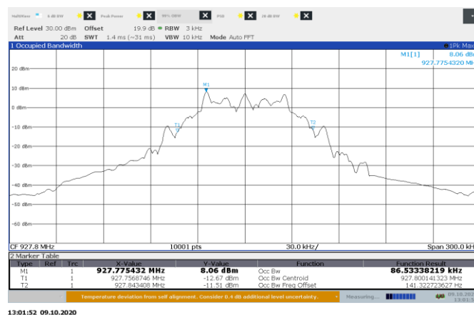
Figure 8.5-6: 99% OBW bandwidth on high channel, 50 kbps
