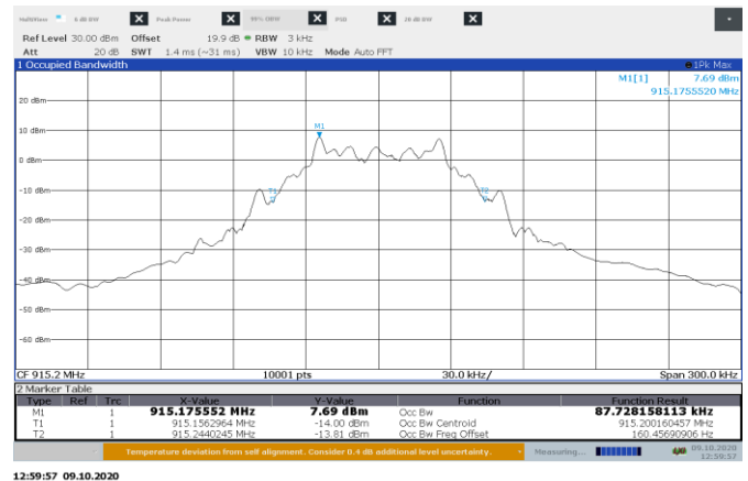
Figure 8.5-5: 99% OBW on mid channel, 50 kbps
