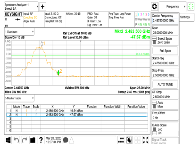
Band Edge_BLE 125k_LowCH00-2402MHz
