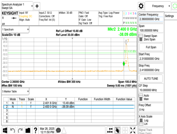
Band Edge_BLE 500k_HighCH39-2480MHz
