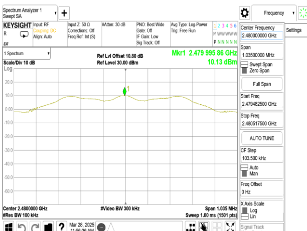
Reference Level_BLE 125k_HighCH39-2480MHz
