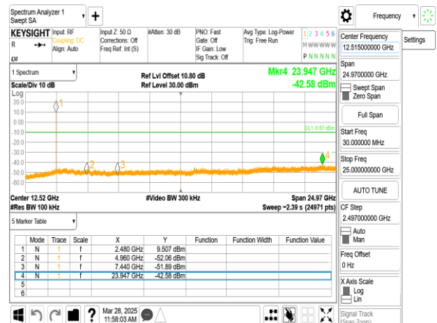
Spurious Emission_BLE 500k_LowCH00-2402MHz
