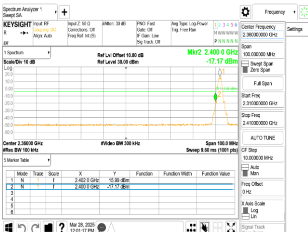
Band Edge_BLE 2M_LowCH00-2402MHz
