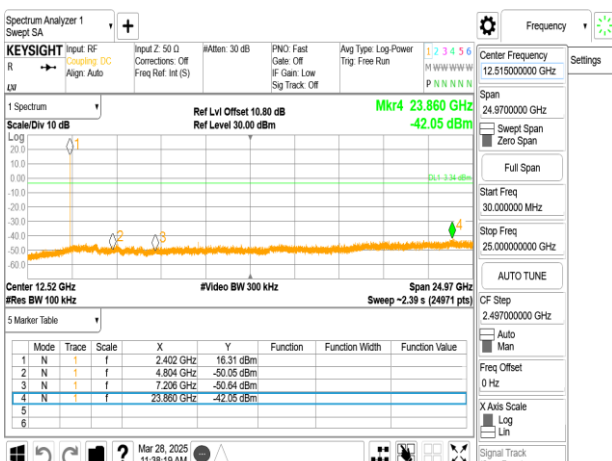
Spurious Emission_BLE 1M_LowCH00-2402MHz
