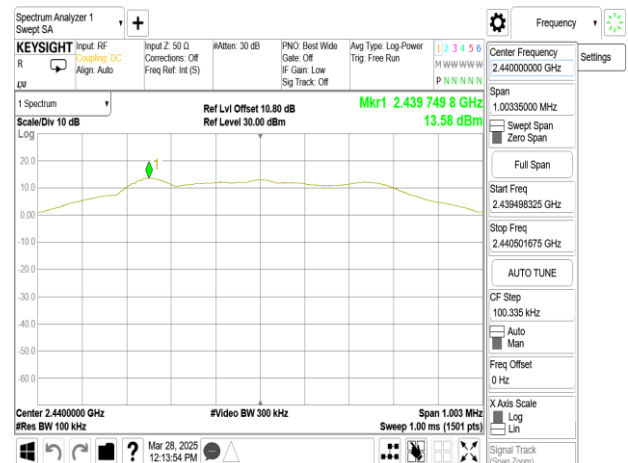
Reference Level_BLE 500k_HighCH39-2480MHz
