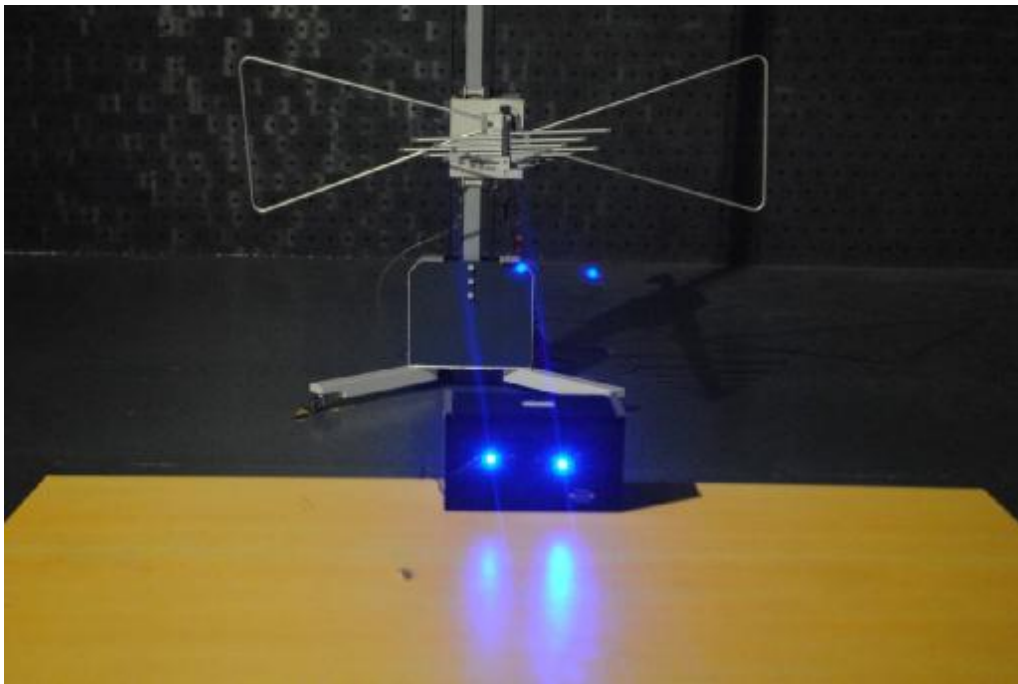
Radiated Emission test view(Frequency from 30MHz to 1GHz)
