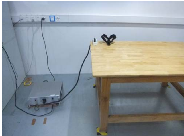
Conducted Emissions Test Setup Front View
