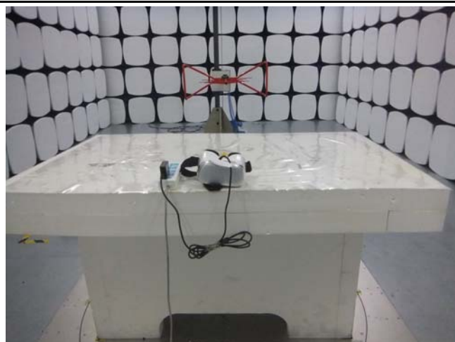
Conducted Emissions Test Setup Front View
