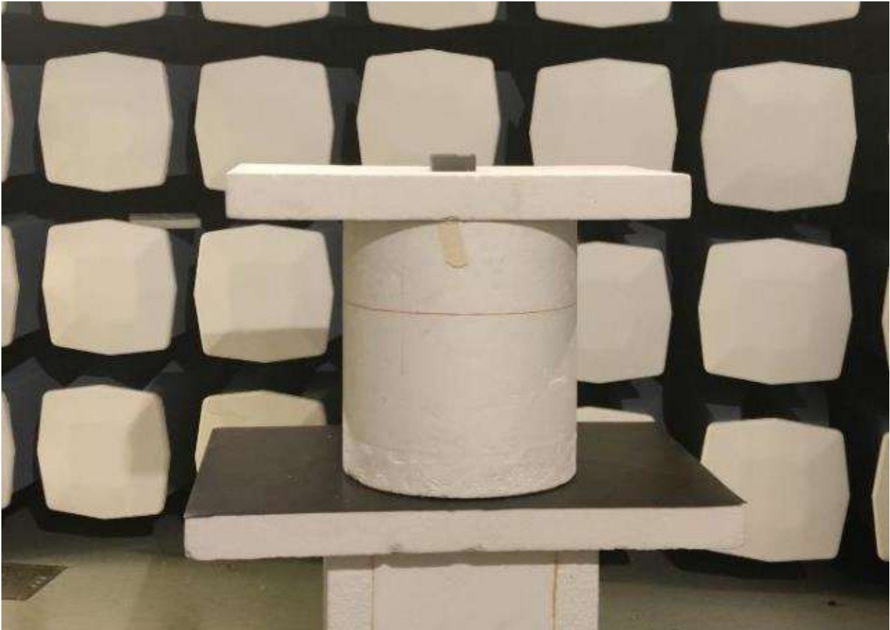
Picture 5 Radiated test setup, Front view, 1-18GHz
