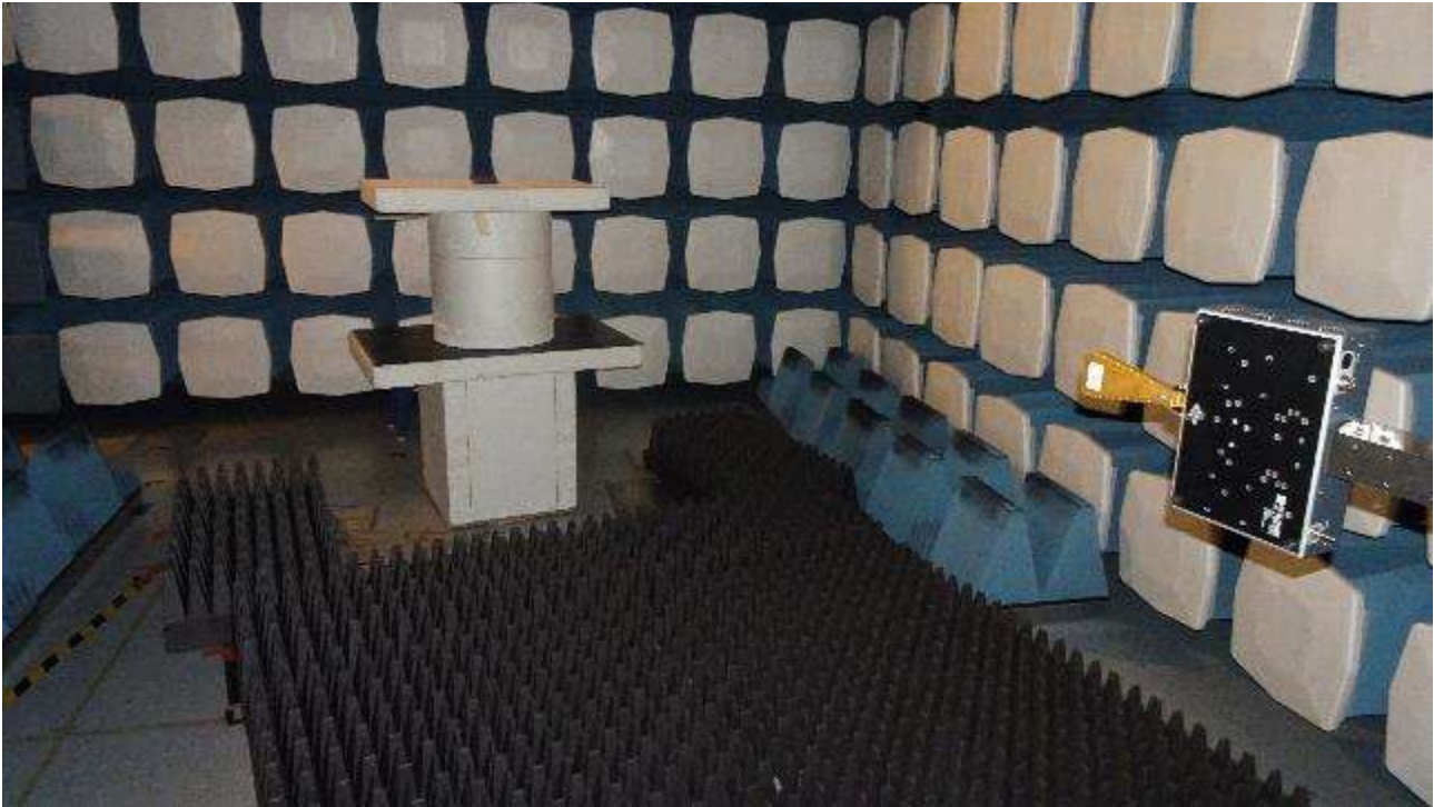
Picture 7 Radiated test setup, Common view, 18 - 26GHz
