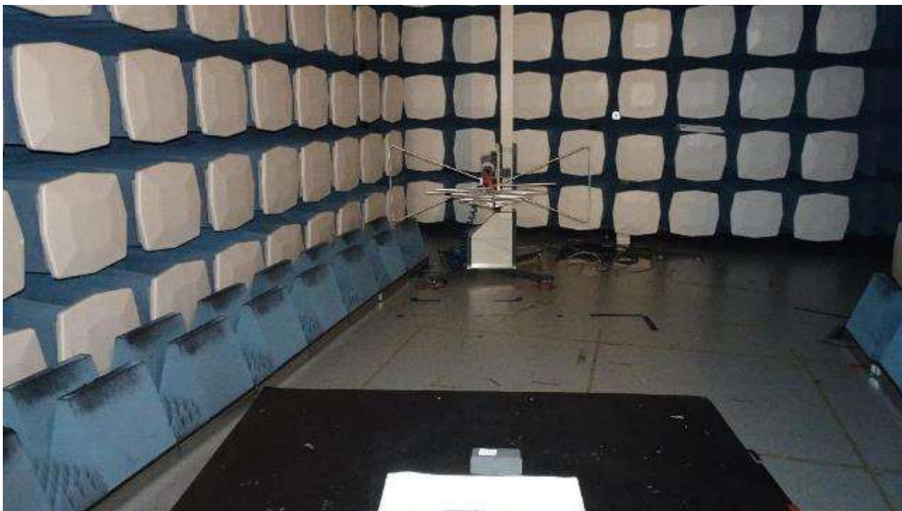
Picture 3 Radiated test setup, back view, 30 – 1000MHz
