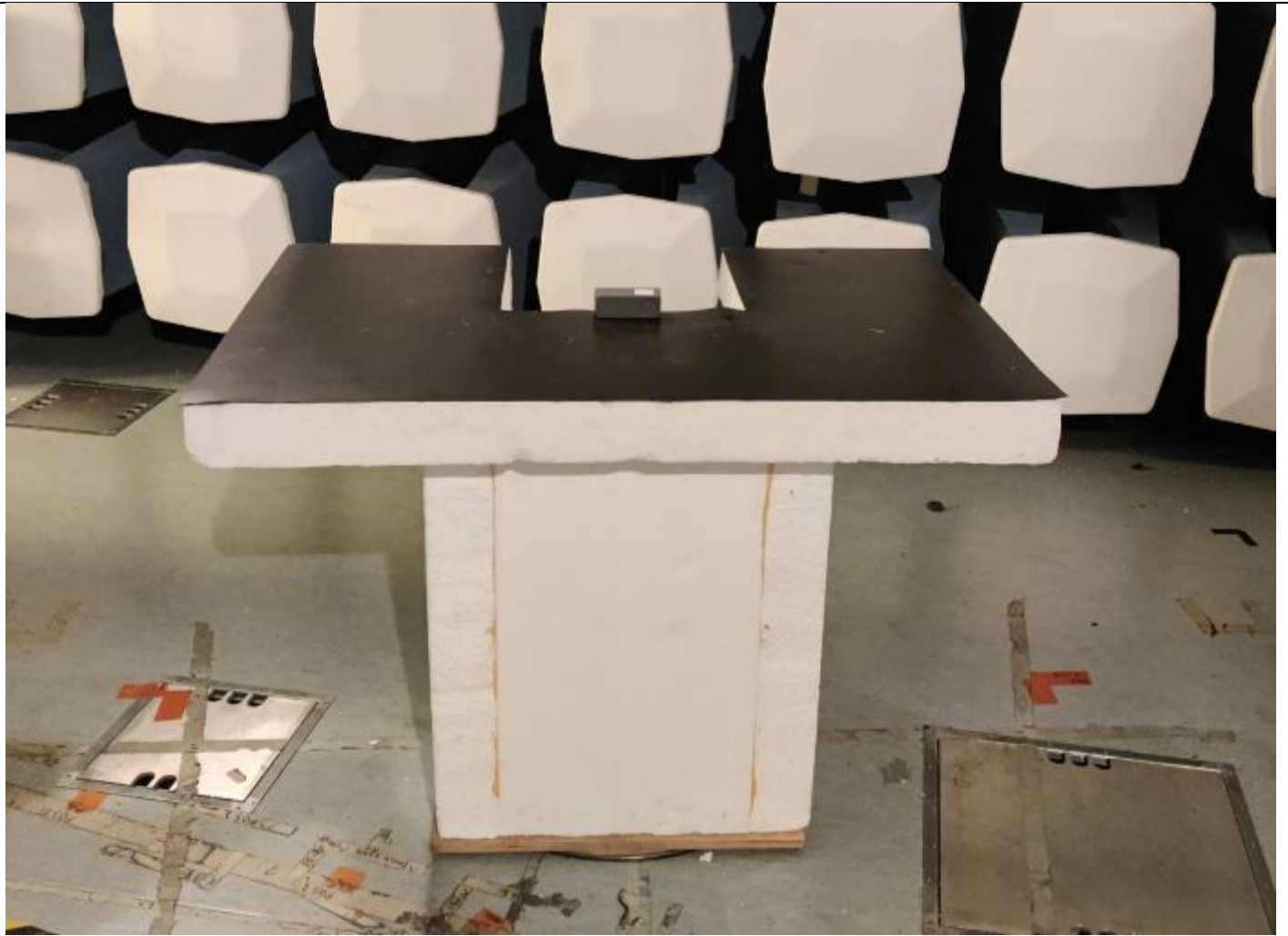
Picture 10, Radiated Spurious Emissions, EUT setup, TX and RX 30 – 1000 MHz
