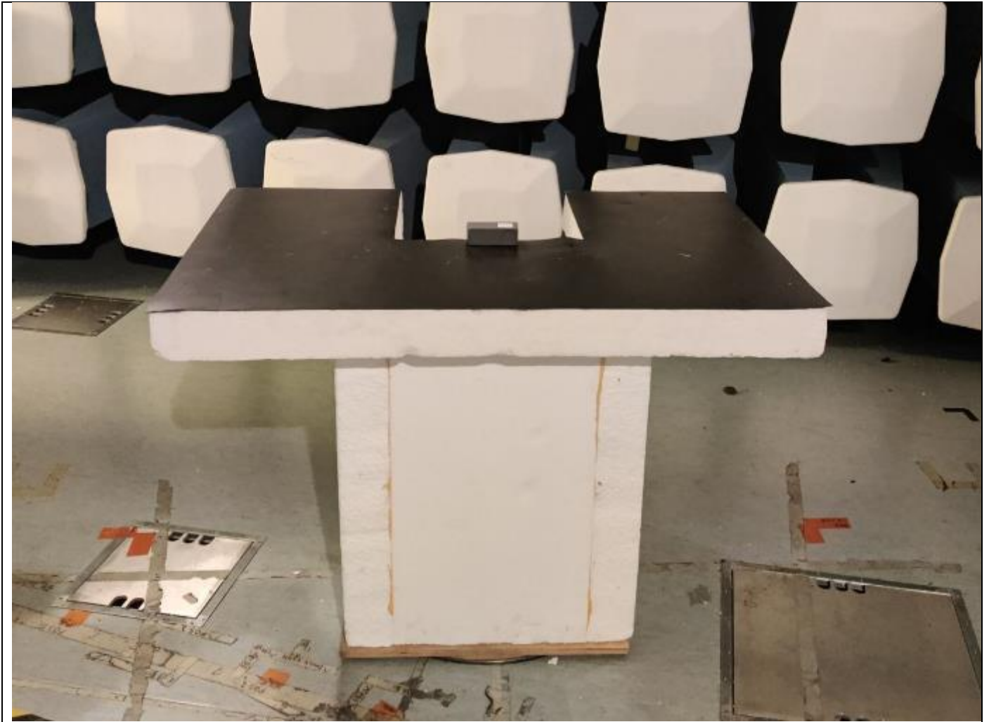
Picture 12, Radiated Spurious Emissions, EUT setup, RX 1 – 18 GHz
