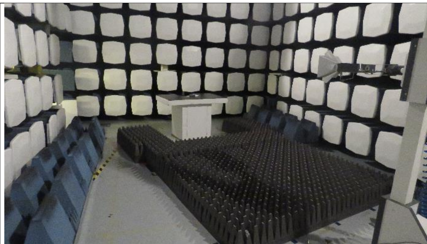
Picture 9, Radiated Spurious Emissions, common setup, RX, 1 – 18 GHz
